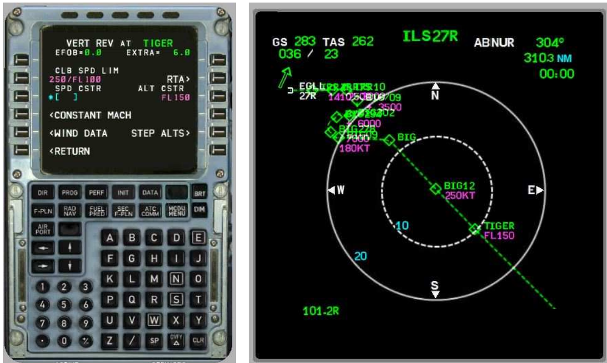
Altitude (below the line ALT CSTR) and speed constraints (below the line SPD CSTR, empty in this example) can be programmed at any waypoint in the flightplan. They are displayed in magenta on both the MCDU-display as well as the navigation display (e.g. flight level 150 at waypoint "TIGER" and 250 knots at waypoint "BIG12"). The FMS calculates its three dimensional flight path in order to respect all constraints as long as aerodynamically possible.
