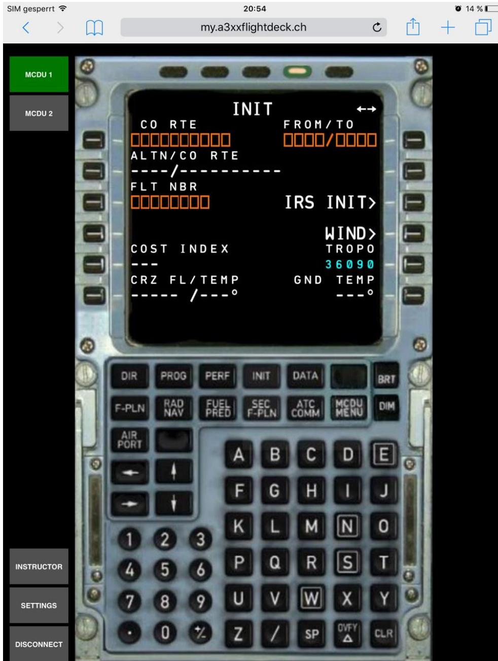
When you type in the scratchpad on your iPad you should see the input simultaneous in your FlightDeck MCDU
